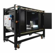
**EZ-Access** is a modular shielded cabinet, ideal for use in universities, research laboratories and NDT test facilities. The **EZ-Access** cabinet's novel door
