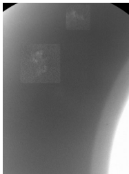
Steel casting with enhanced regions of porosity
