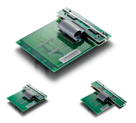
X-Card | The X-Card detector card is a dual-energy linear array X-ray detector card. It has two two-layers of Silicon photodiode arrays, targeted for different X-ray energy ranges. X-ray sensitive scintillant material is located on top of the photodiode arrays to convert X-ray signal in to visible light, which generates current at photodiode. The electrical current signals from photodiodes are connected to inputs of chargesensitive preamplifier array ASICs.
